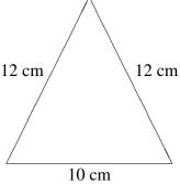
To find the area, we need to find the vertical height. We cannot use Pythagoras in the original triangle since it is not right-angled. We must use its line of symmetry to create a right-angled triangle, as shown.
